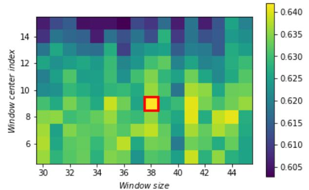
**Fig.5** Cross-validation score using only speeds with a multi-layer perceptron model using one layer
