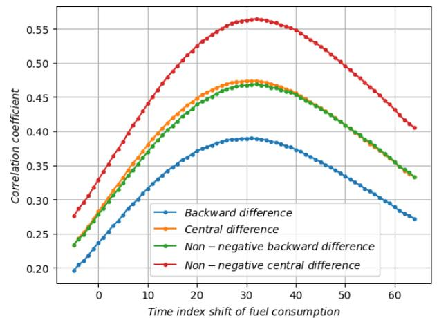
**Fig.1** Correlation between various forms of accelerations and fuel consumption
