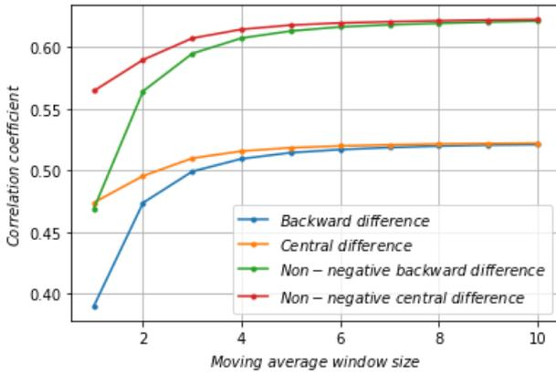
**Fig.2** Maximum correlation between various moving averaged accelerations and fuel consumption
