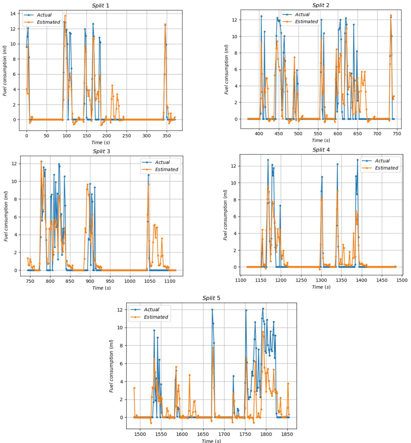
Fig.7 Actual and estimated fuel consumption using the best MLP model for each cross-validation split
